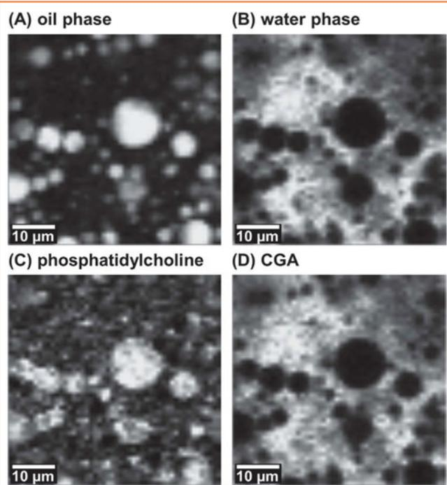
**Figure 4.** Raman distribution maps of the test substance 4 containing the liposomal loaded fraction C showing the local distribution of (A) the oil phase, (B) the water phase, (C) phosphatidylcholine and (D) CGA.
