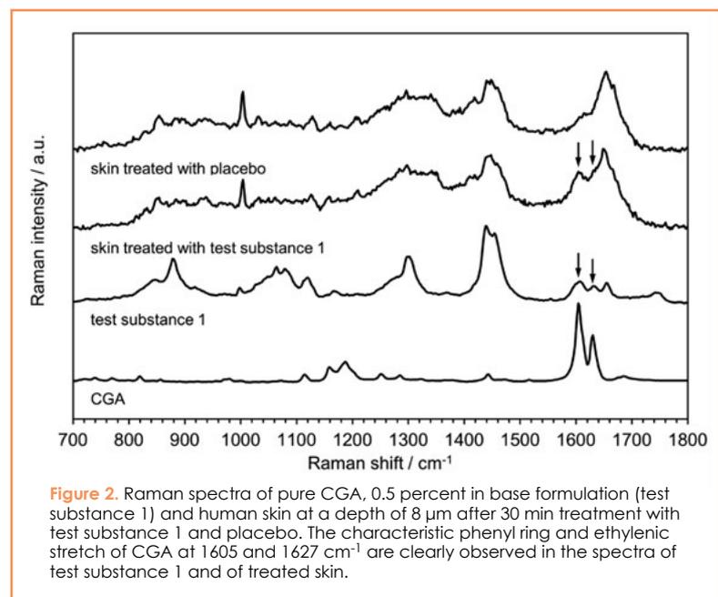
that had been applied to the volunteers. Figure 2 shows also a typical Raman spectrum of skin before and after treatment with the test substance at a skin depth of 8  $\mu\text{m}$ . The alterations in the spectrum due to the presence of CGA are clearly observed.
