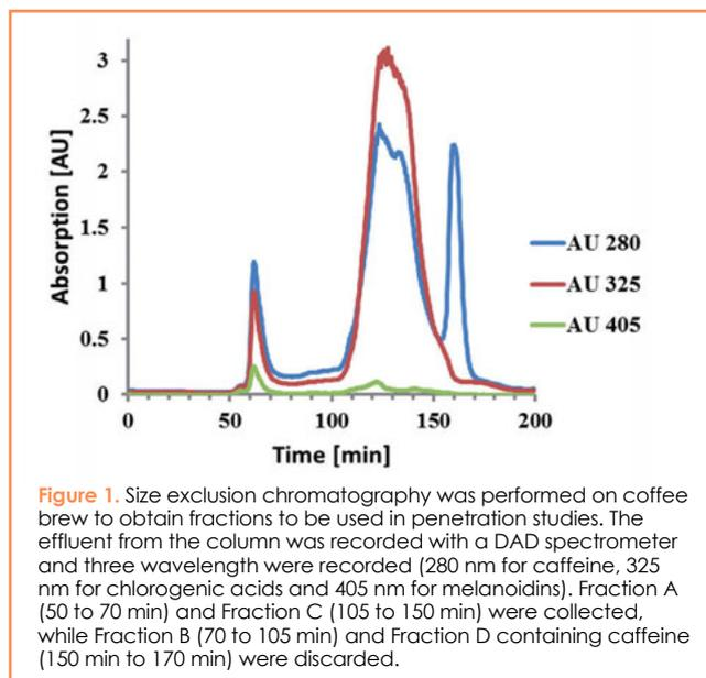
**Figure 1.** Size exclusion chromatography was performed on coffee brew to obtain fractions to be used in penetration studies. The effluent from the column was recorded with a DAD spectrometer and three wavelengths were recorded (280 nm for caffeine, 325 nm for chlorogenic acids and 405 nm for melanoidins). Fraction A (50 to 70 min) and Fraction C (105 to 150 min) were collected, while Fraction B (70 to 105 min) and Fraction D containing caffeine (150 min to 170 min) were discarded.
